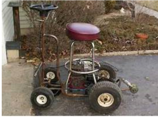
Kile Wygle's bar stool, which is powered by a deconstructed lawn mower.
